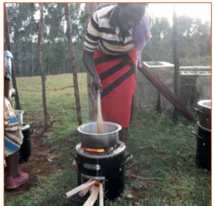
Field testing of stick-fed rocket stove
