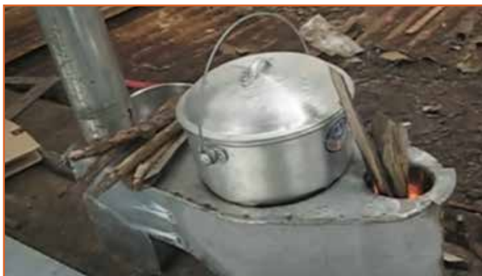
Gravity stick-fed rocket stove
